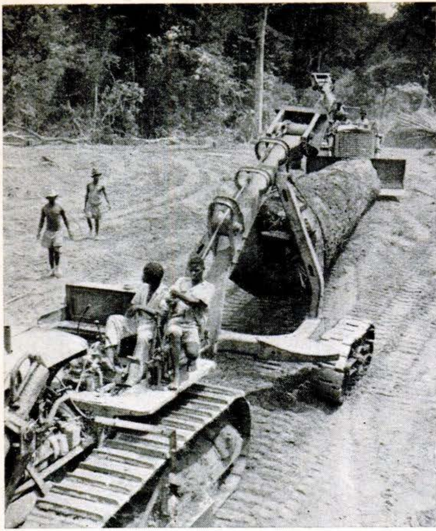
TWO TRACTORS , one dragging and another pushing, are needed to move big logs out of the jungle to a clearing. The log hangs from a hoist attached to the tractor in foreground.
